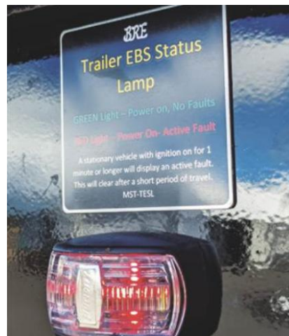
Figure 4. Trailer EBS Status light fitted to outer side of trailer in between chassis rails. Labelling used, one light with multi-colours solution
