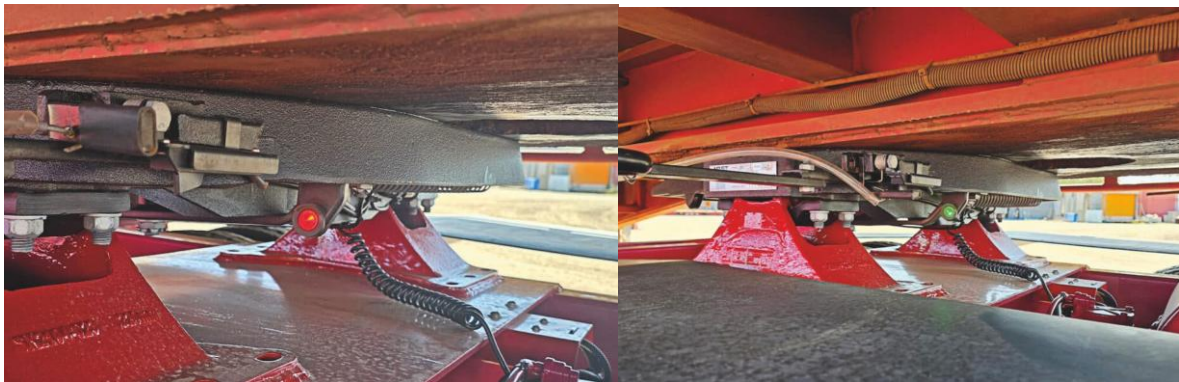
Figure 10. Fifth wheel locking status indicator light
