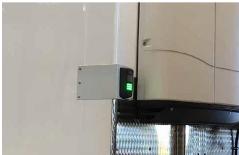
Figure 6. Example of Refrigerator status light on trailer
