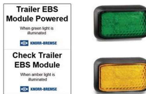
Figure 4. Trailer EBS Status light fitted to outer side of trailer in between chassis rails. Labelling used, one light with multi-colours solution
