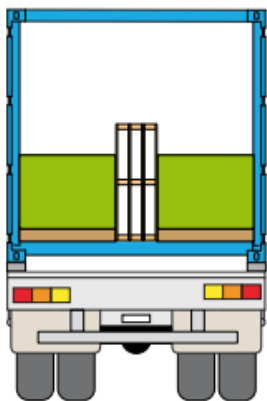
Gap filled with pallets
