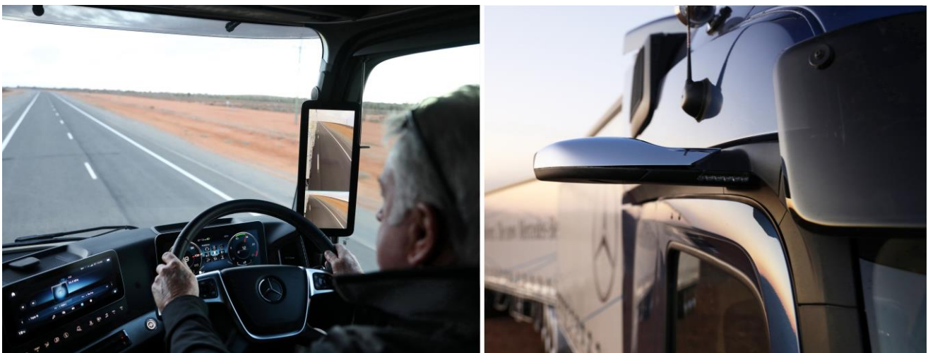
Figure 2 – An internal monitor (left) and external camera (right) of a camera-monitor system for indirect vision (source: supplied by Daimler Truck and Bus Australia Pacific)
