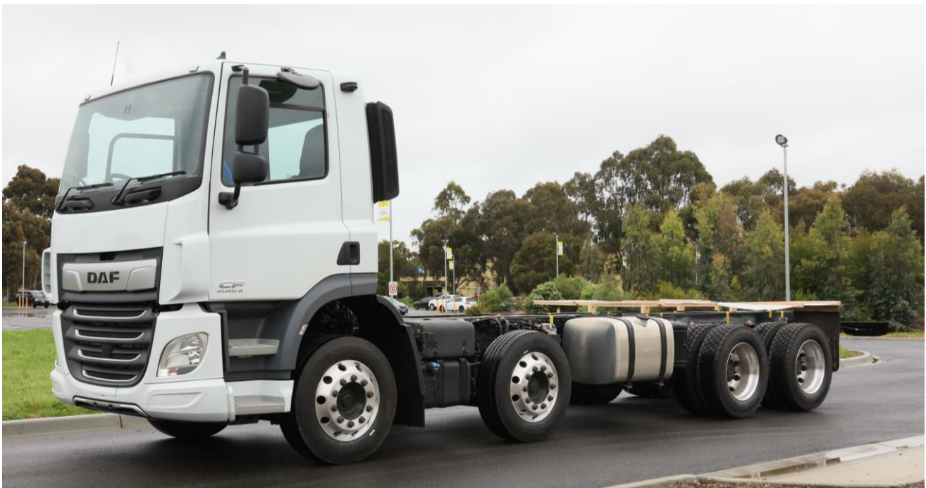
Figure 5 – A heavy rigid truck (cab-chassis) with a twin steer axle group (source: supplied by Paccar Australia)
