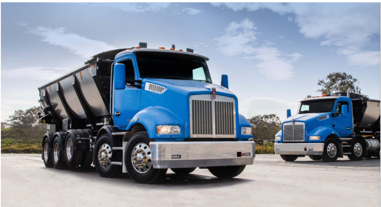
Figure 6 – A heavy rigid truck with a leading retractable axle (source: supplied by Paccar Australia)
